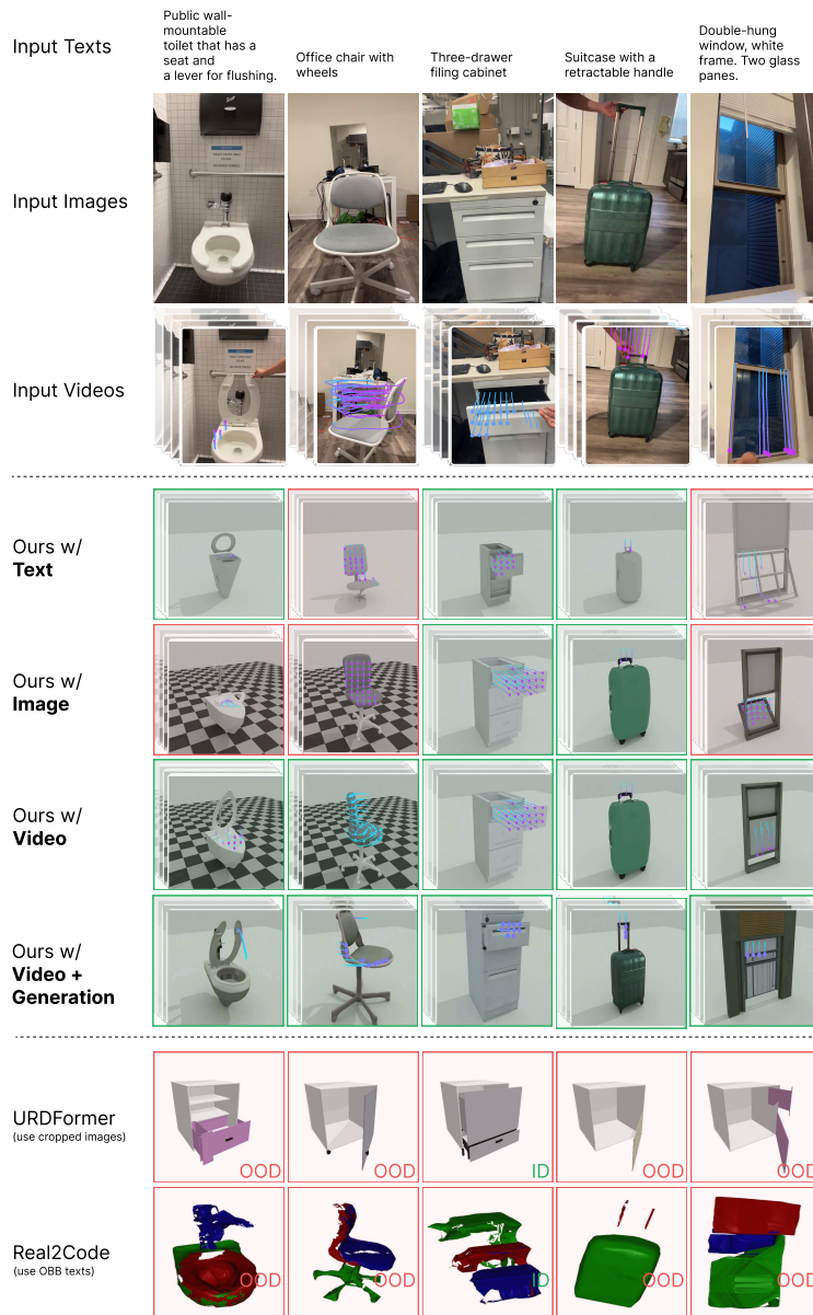
Figure 7: In-the-wild Reconstruction. We demonstrate ARTICULATE-ANYTHING’s performance input modalities compared to prior works URDFormer and Real2Code. Green and red borders denote correct and incorrect predictions with respect to the input videos. Our simulated videos are generated by varying joint limits and annotated with Cotracker. Casual inputs: Our video-based approach excels with casually captured inputs in cluttered environments while baselines require extensive manual curation (more details in Appendix A.4 Fig. 17 and 18). Ambiguous articulation: Interestingly, our video-based method can resolve ambiguities in static inputs (e.g., chair rotation vs. height adjustment, window sliding vs. tipping). Baseline limitations: URDFormer consistently predicts drawer-like structures and is sensitive to minor misalignments (e.g., slightly tilted drawers). Real2Code, which uses multi-view images for mesh reconstruction and text-oriented bounding boxes (OBBs) for joint prediction, achieves good global alignment from DUST3R but produces low-quality 3D segmentation using a finetuned SAM, leading to joint prediction errors. We also included some results using a mesh generation model instead of retrieval to allow for even more customized asset creation with more details in Appendix A.8. Mesh reconstruction quality result is included in Tab. ?? in Appendix A.6. Please visit our website for additional demos: https://articulate-anything.github.io/ .
